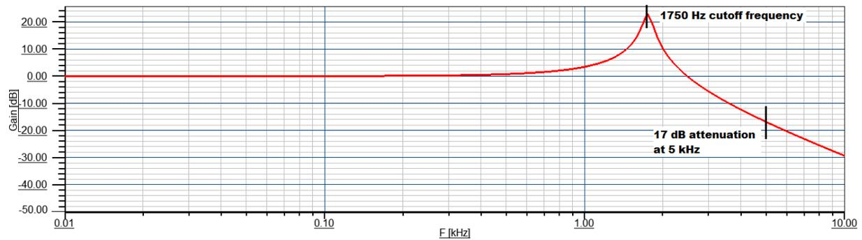
Figure 9 Typical 5 kHz LC filter frequency response
