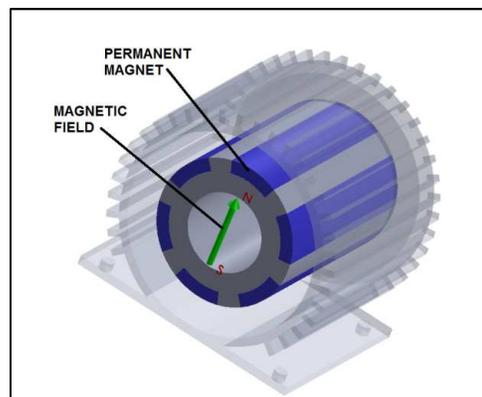
Figure. 5 PM motor rotor illustration
