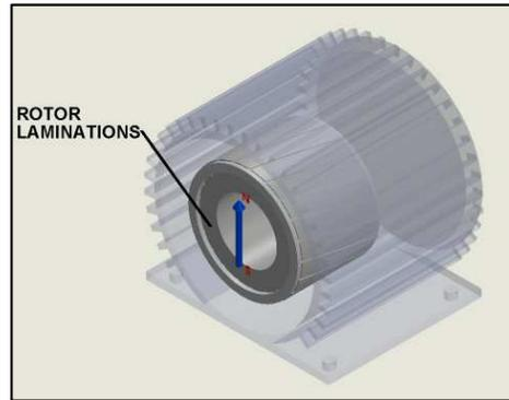
Fig. 4 Rotor laminations
