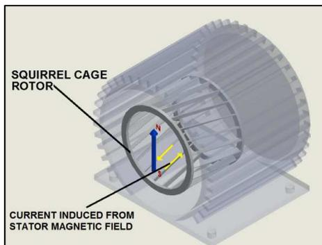
Figure. 3 Squirrel cage rotor and induced currents from stator
