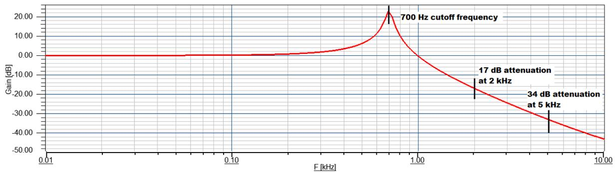
Figure 8 Typical 2 kHz LC filter frequency response
