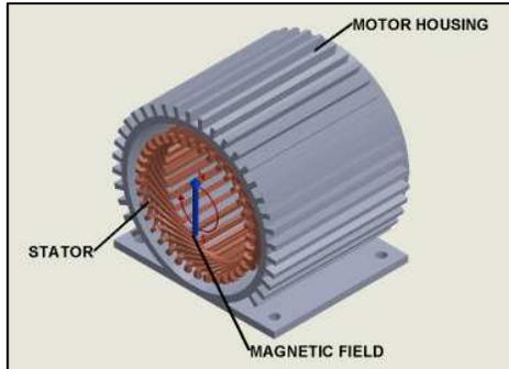
Figure 1 Stator windings and motor housing
