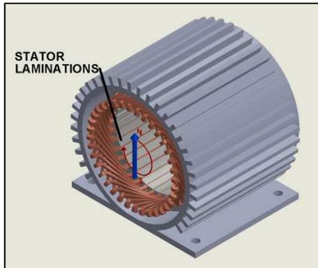
Figure. 2 Stator windings, motor housing and stator laminations
