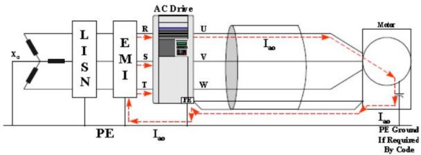
EMC filters are designed so that circuit values for L and C are optimized for lowest power at the fundamental utility frequency and still be able effectively attenuate 50 KHz . The resultant design usually has a high reactive component to its impedance and will be critically damped at about 0.707.
