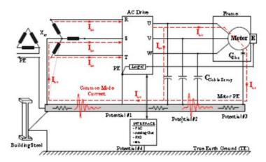
There are two main reasons for employing EMC input filters, namely: (1) to prevent electromagnetic interference of the offending VFD with electronic systems present in the neighboring environment, (2) Governing regulating bodies responsible for policing power quality mandate the installation of appropriate EMC filtering especially in Europe.
