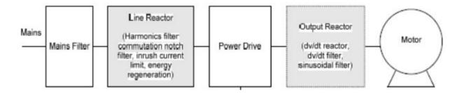
For VFD's that have built in EMC filters and will be used with either a reactor or Matrix filter MTE recommends disabling the drives built in EMC filter or using a drive that does not have a built in EMC filter and adding a separate EMC filter connected to the utility as shown above.
