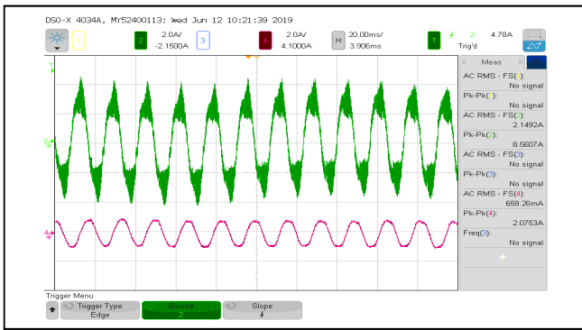
Fig. 20. CM Currents before and after using 45A filter
