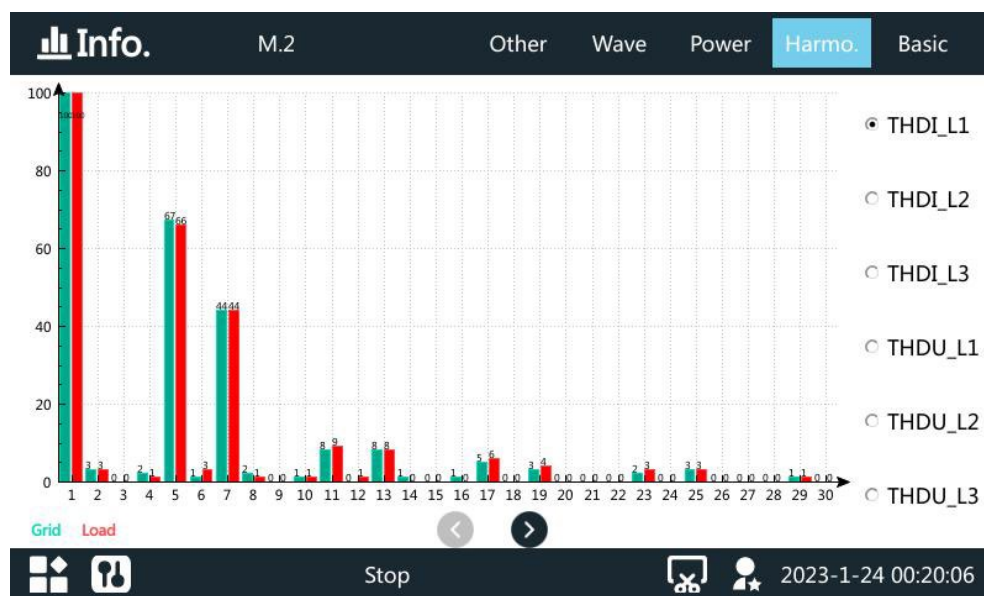
Figure 3-19: Example Harmonic Spectrum
