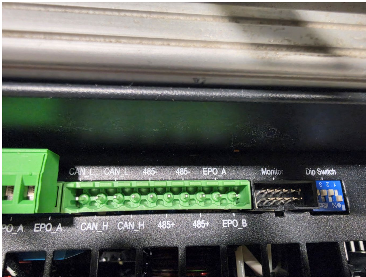
Figure 3-3: Rear signal panel communication terminals
